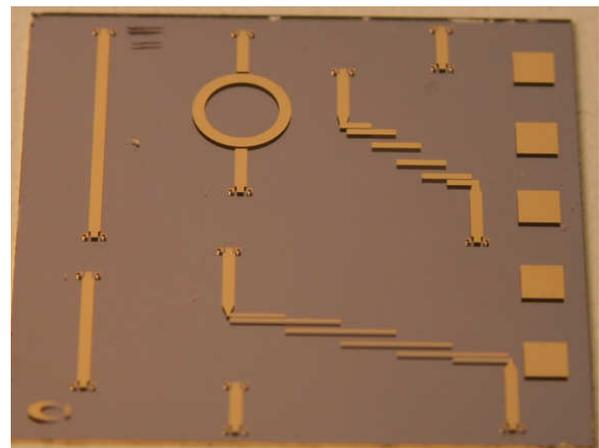
**Figure 6 AQ1 Fabrication Coupon of RF Components**
