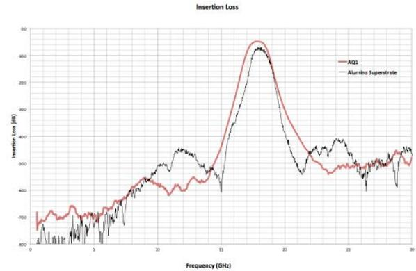
**Figure 9. Measurement results of the 18GHz filter for AQ1 and Alumina Superstrate**
