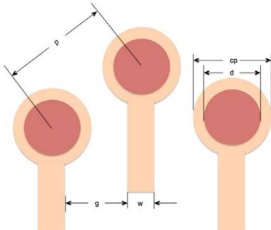
**Figure 4. Design parameters for traces and vias**
