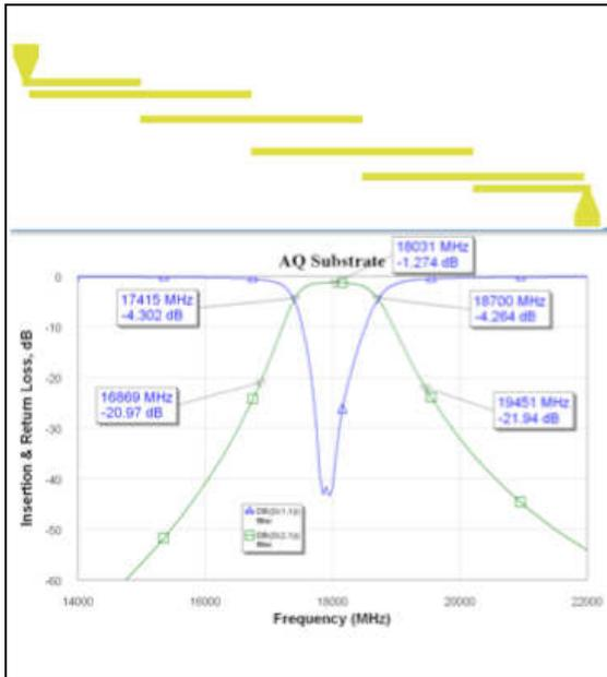
**Figure 8. 18GHz Filter design on AQ1**
