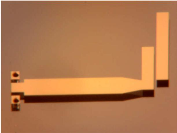
**Figure 7. RF Feed line showing the ground vias**
