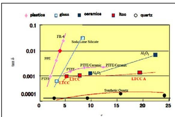
Figure 2. Loss tangent data for board/package materials.
